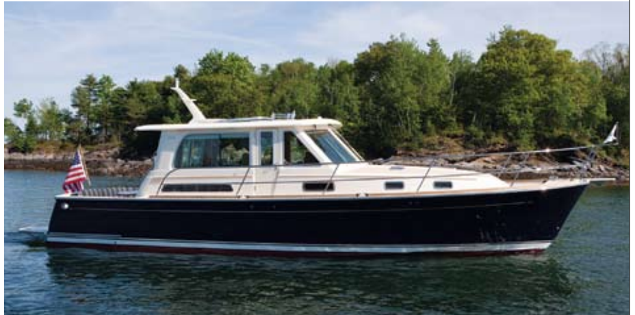
SIBLING RIVALRY: The new 40 reflects the styling of the successful 52, with enough tumblehome to please the eye, while not compromising cockpit volume. A flying bridge is available.
